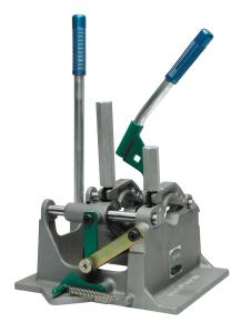
The 2LC will butt fuse ½ CTS to 2" IPS (16mm to 60mm) pipe. By employing a semi-automatic locking cam (LC) system, the 2LC expertly maintains force during the cooling cycle.
