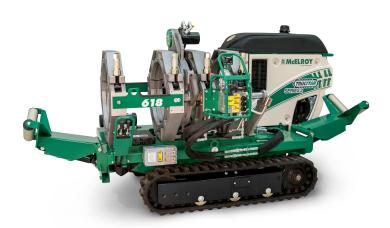
The TracStar <sup>®</sup> 618 Series 2 has been completely redesigned based on feedback that came directly from the field. The new machine now shares a common vehicle with the 28, 250, and 412 range of TracStars and is powered by a powerful diesel engine - which is especially useful on jobsites where gasoline is not permitted.
